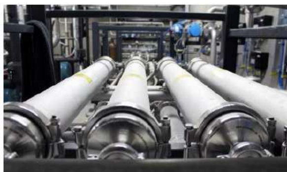
Membranes modules in a container
